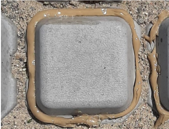
Photo 7: Option 1 Adhesive Application
