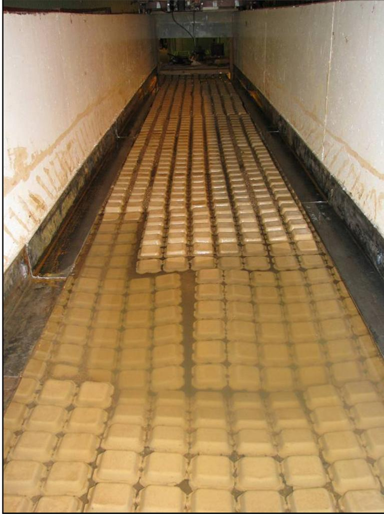
**Figure 3-4: Drivable Grass<sup>®</sup> system following final test of Configuration 2 (Test 4)**
