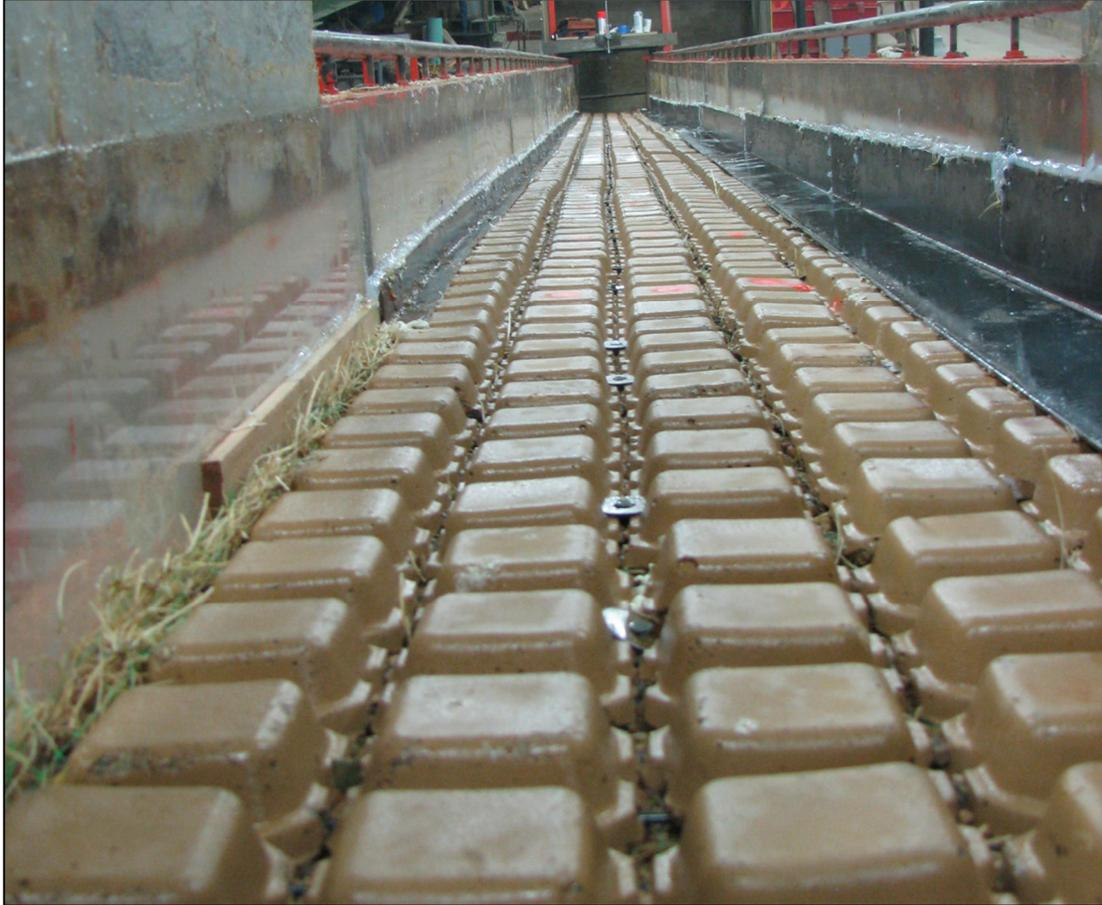
**Figure 3-10: Drivable Grass<sup>®</sup> system following final test of Configuration 5 (Test 40)**
