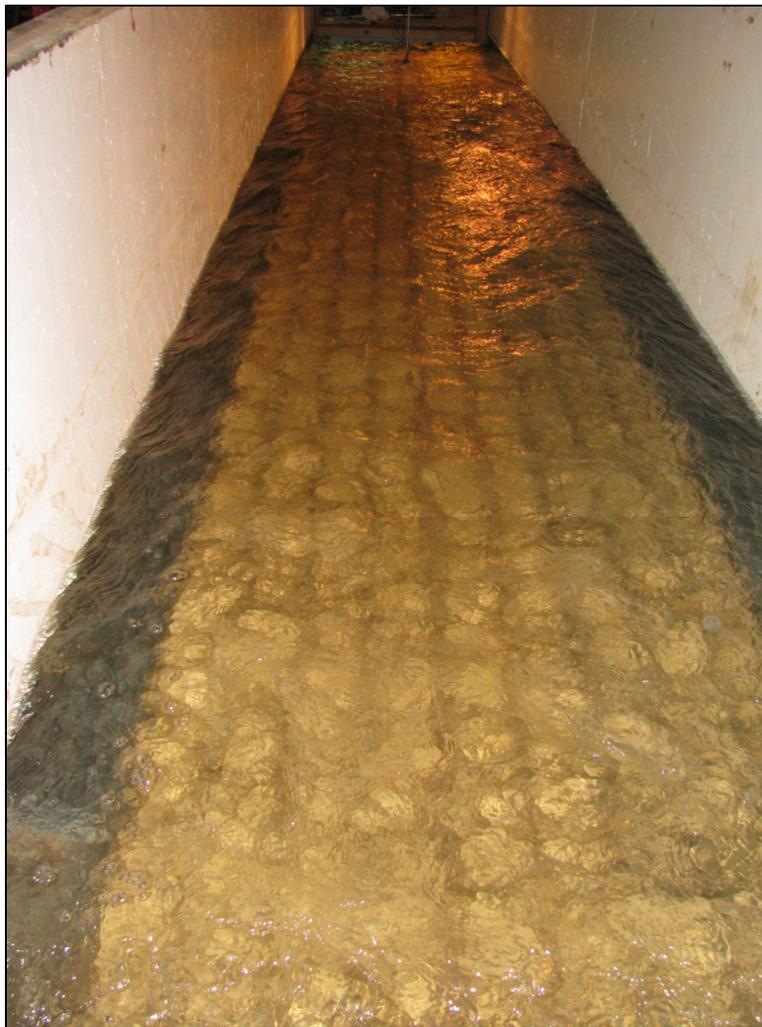
**Figure 3-1: Drivable Grass<sup>®</sup> system during Test 1 (Configuration 1)**
