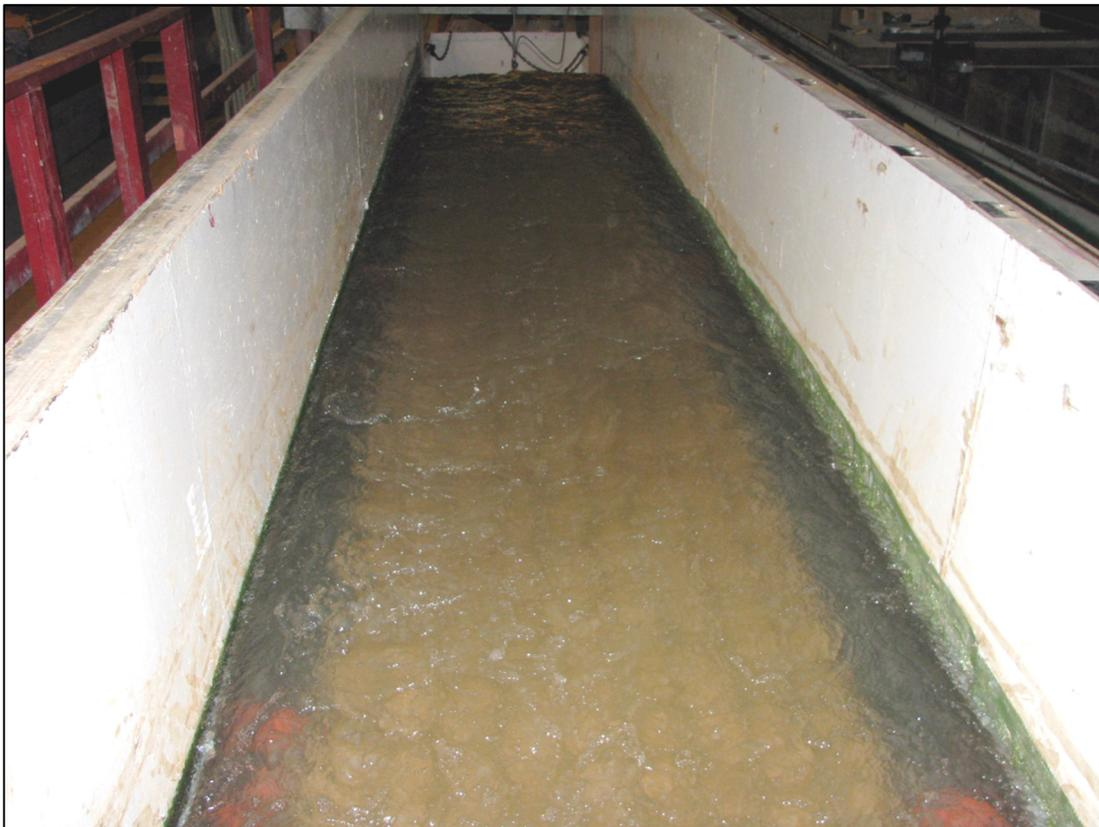
**Figure 3-7: Drivable Grass<sup>®</sup> system during Test 30 (Configuration 4)**
