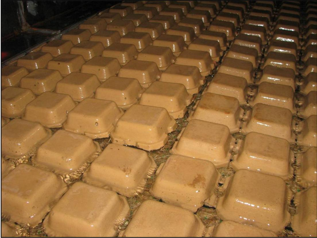
**Figure 3-6: Drivable Grass<sup>®</sup> system following final test of Configuration 3 (Test 20)**
