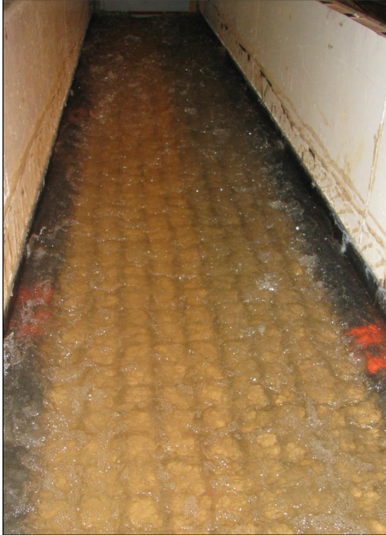
**Figure 3-5: Drivable Grass<sup>®</sup> system during Test 19 (Configuration 3)**
