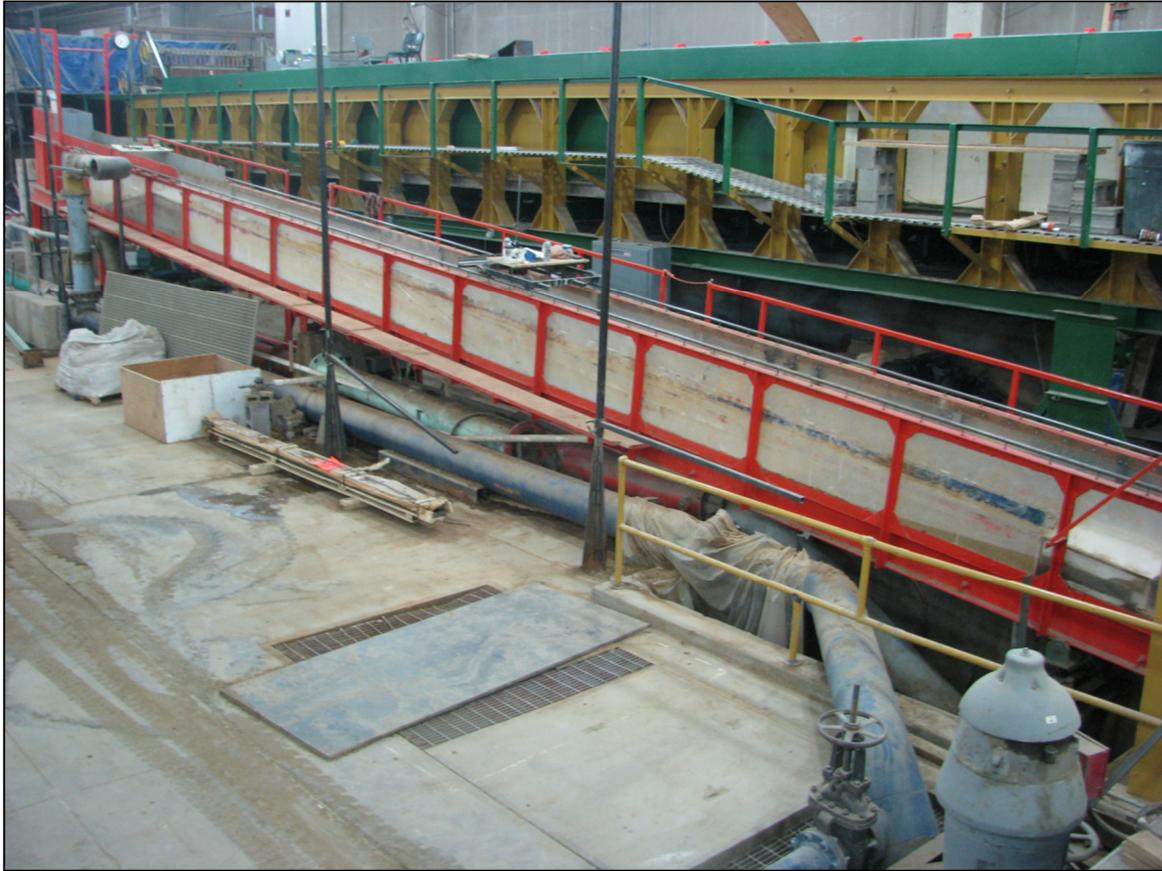
**Figure 2-3: Two-foot wide adjustable-slope flume**
