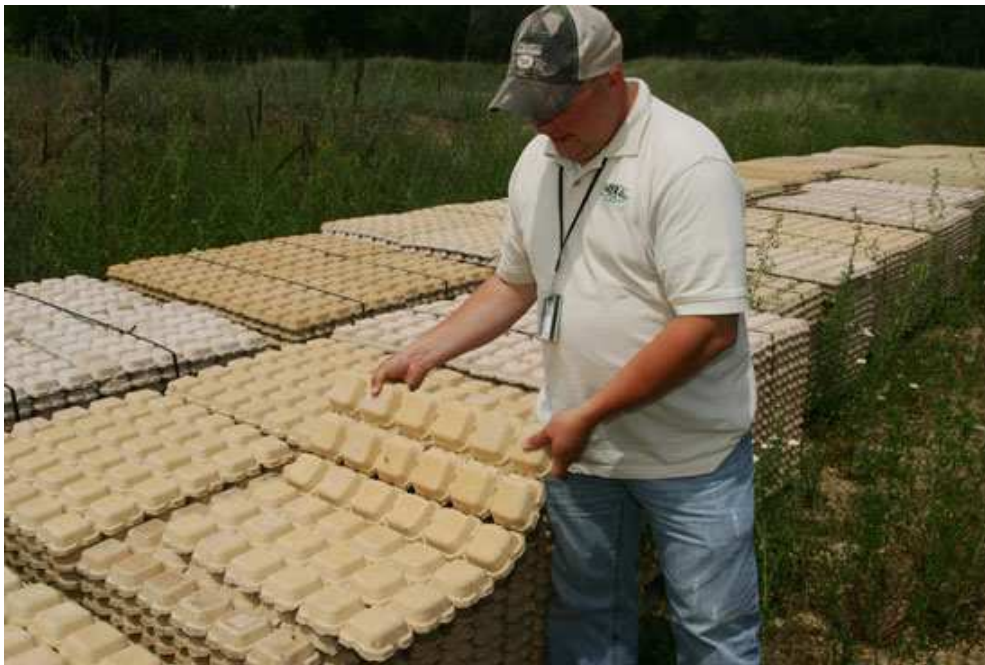
Brooks Lundeen, the Land Rehabilitation and Maintenance (LRAM) coordinator for the Integrated Training Area Management (ITAM) program, checks out a drivable grass pavement system, which is used to improve access for vehicles and equipment in Fort McCoy training areas. (Photo by Rob Schuette)
