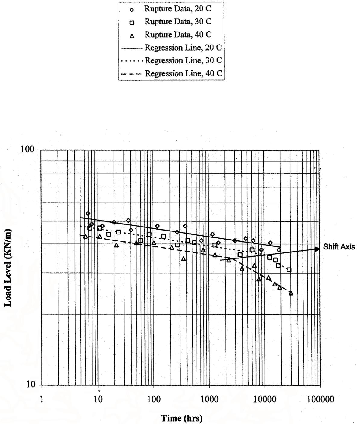
Figure B.6 Stress rupture data for polyolefin geosynthetic.
