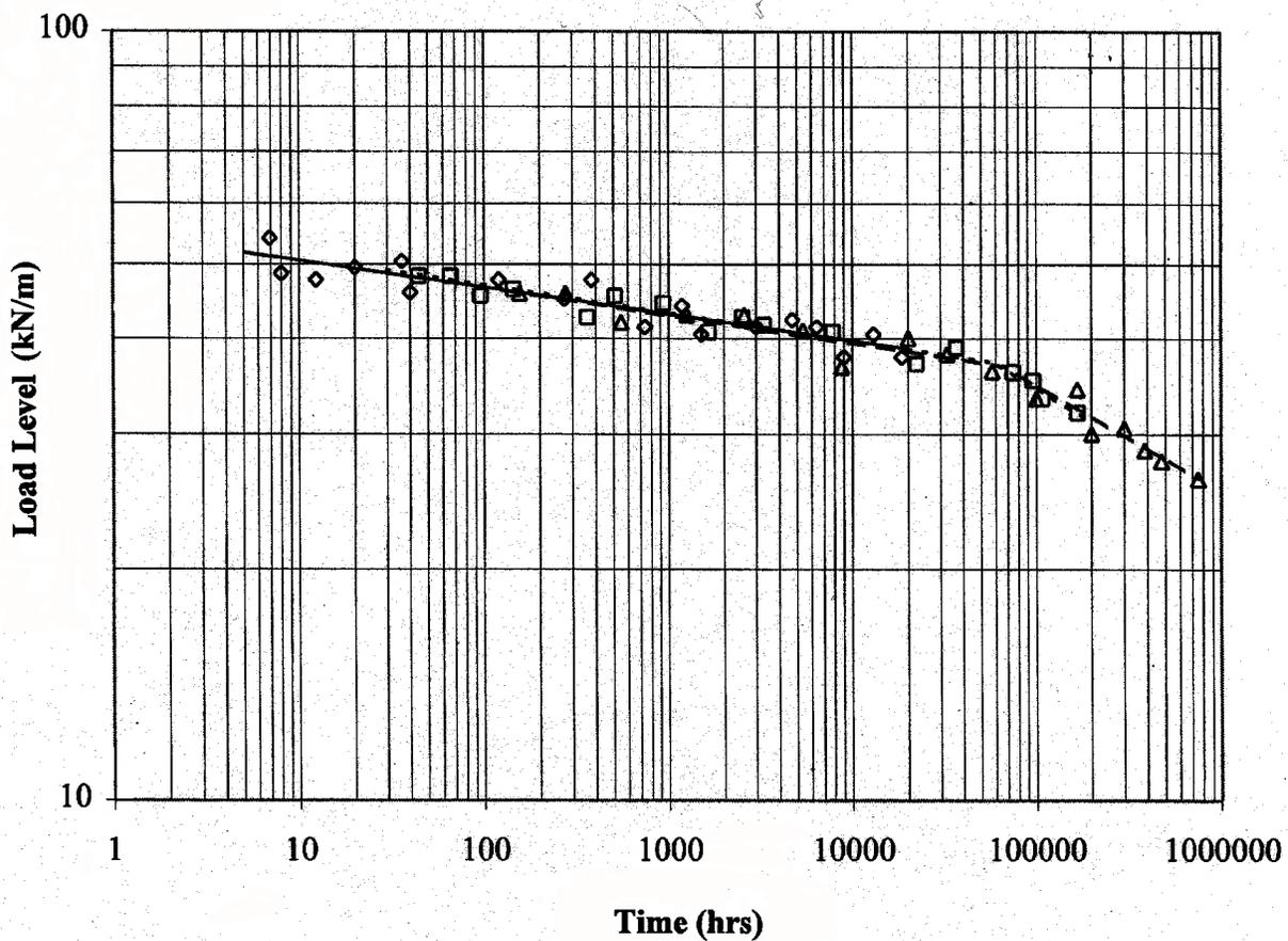
Figure B.7 Stress rupture data for polyolefin geosynthetic after time/load shifting.
