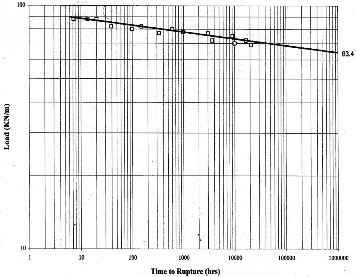
Figure B.4 Stress rupture data for PET geosynthetic at 20°C.
