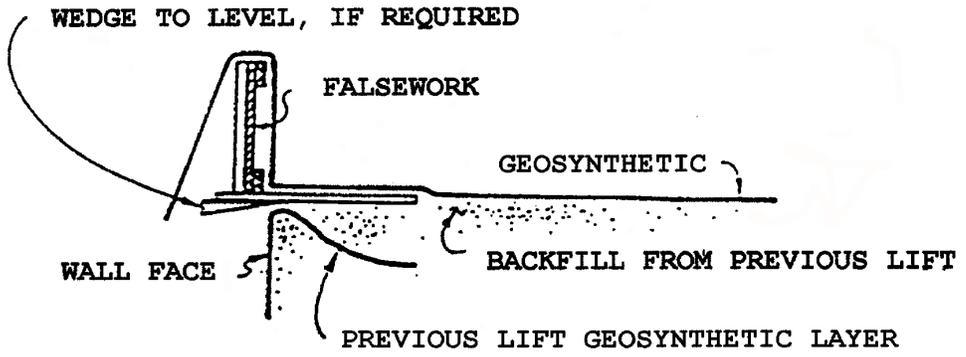
(1) PLACE FALSEWORK AND GEOSYNTHETIC ON PREVIOUS LIFT
