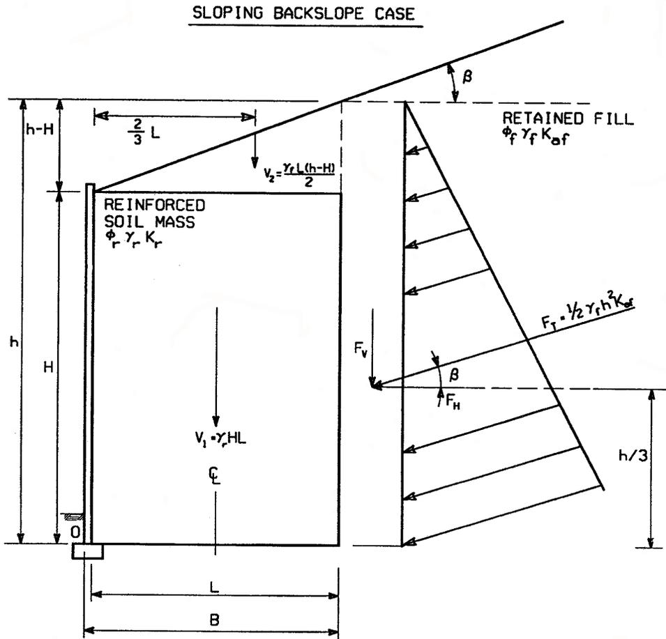
**Note:** For relatively thick facing elements (e.g., segmental concrete facing blocks) it may be desirable to include the facing dimensions and weight in sliding and overturning calculations (i.e. use "B" in lieu of "L").
