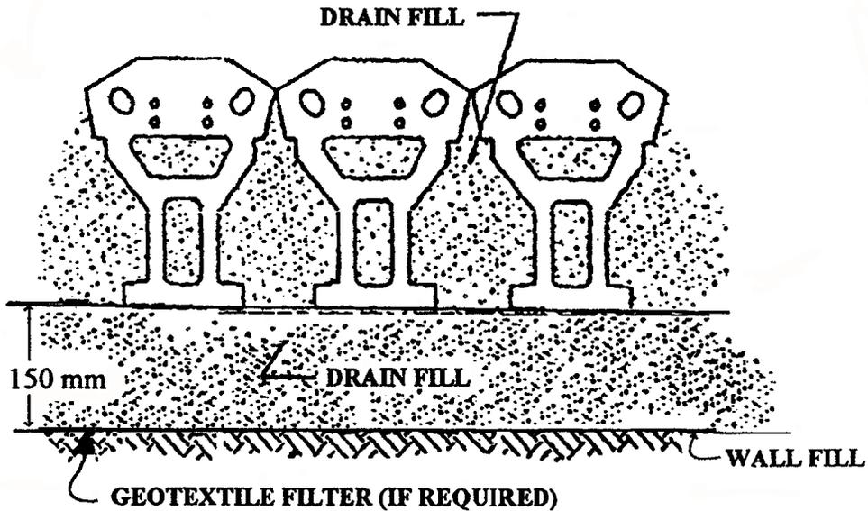
Figure 43. Drain fill placement for MBW with cores or tails.
