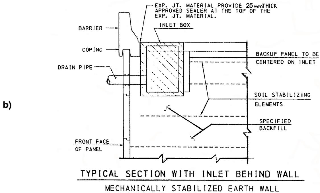
Figure 41. Obstruction details: a) conceptual; b) at inlet.
