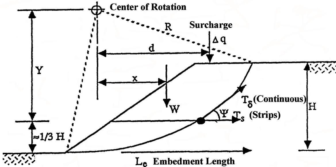
Figure 54. Modified limit equilibrium analysis for reinforced slope design.
