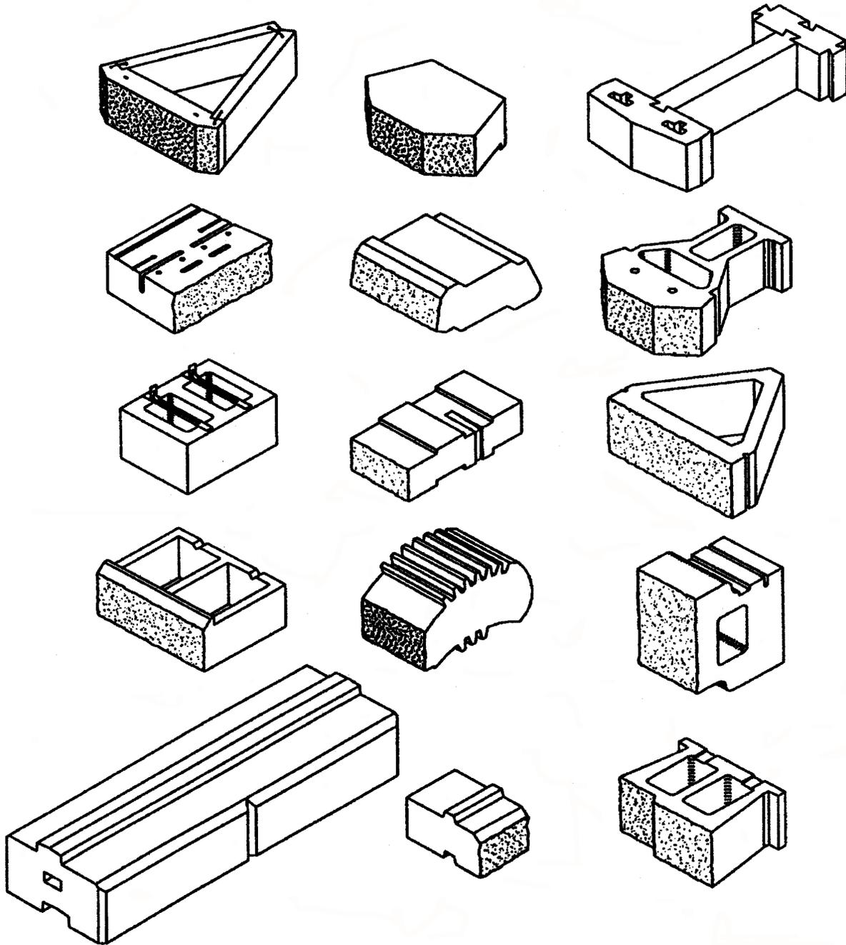
Figure 9. Examples of commercially available MBW units (from NCMA Design Manual for Segmental Retaining Walls).
