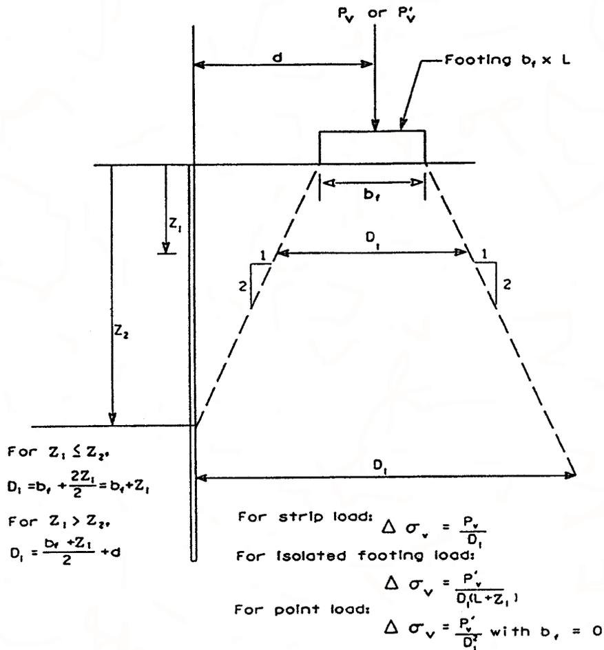
Where:  $D_1$  = Effective width of applied load at any depth, calculated as shown above
