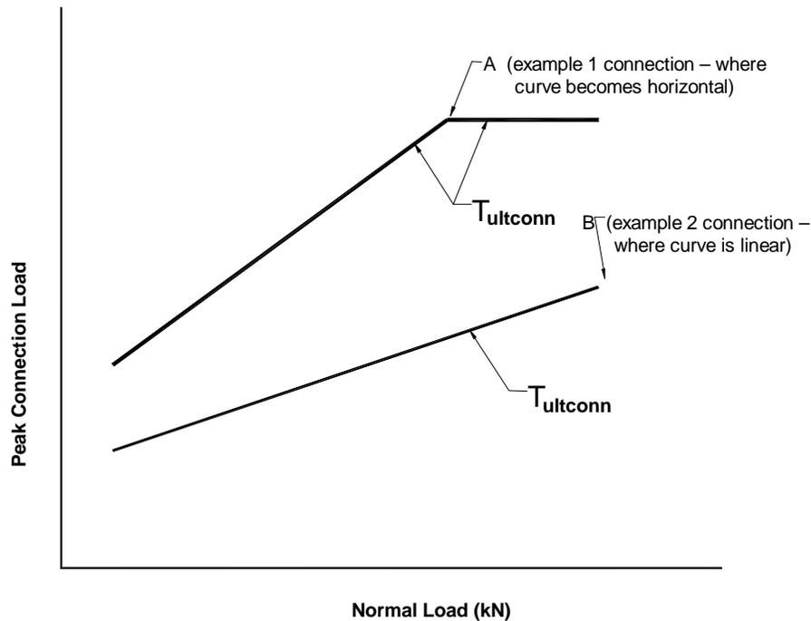
Figure A.3 Connection Strength (NCMA SRWU-1) verses Normal Load
