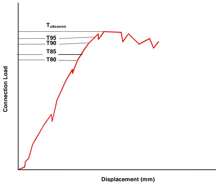
Figure A.4 Connection Strength versus Displacement (NCMA SRWU-1)
