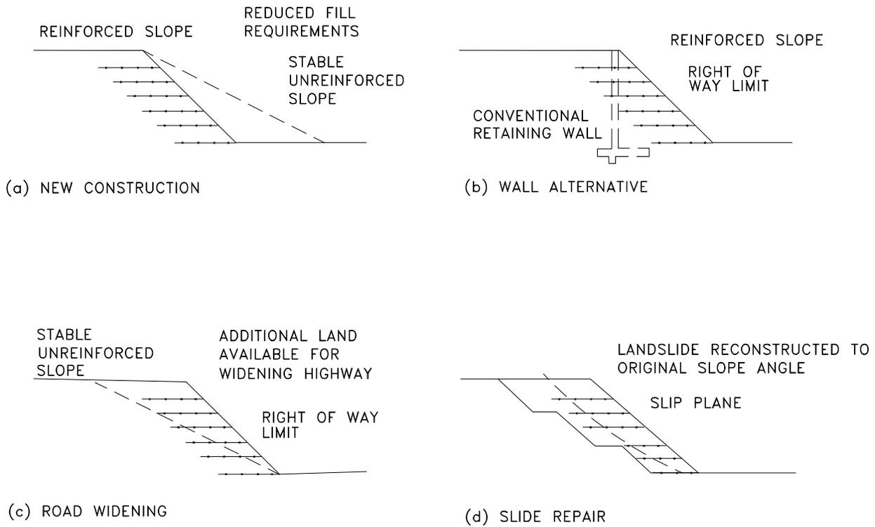
Figure 5. Application of reinforced soil slopes.
