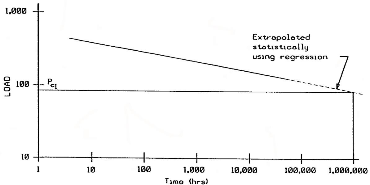
Figure B.2 Extrapolation of stress rupture data and the determination of creep limit load.
