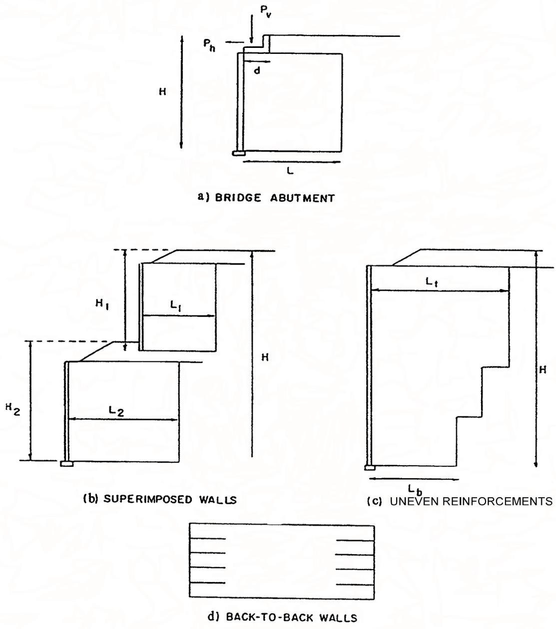
Figure 45. Types of complex MSE structures.
