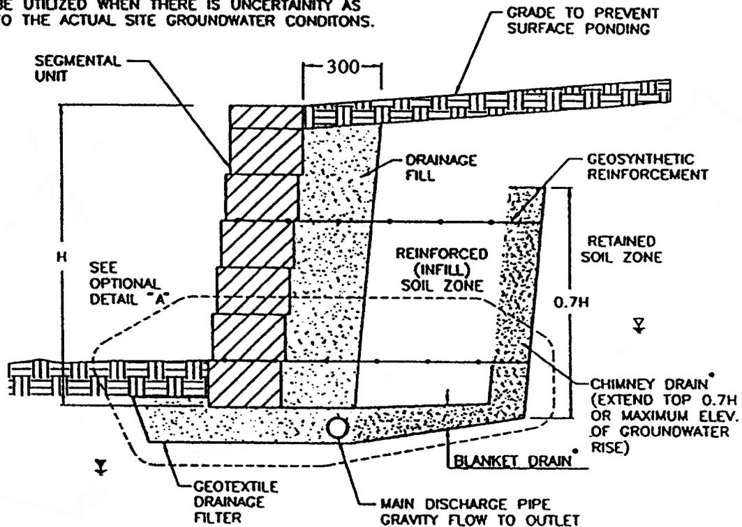
NOTE: CHIMNEY DRAIN AND/OR BLANKET DRAIN MAY BE REPLACED WITH AN APPROPRIATE GEOCOMPOSITE AT THE DISCRETION OF THE WALL DESIGN ENGINEER.
