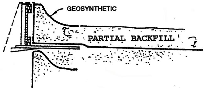
(2) PLACE/COMPACT PARTIAL BACKFILL AND OVERLAP GEOSYNTHETIC
