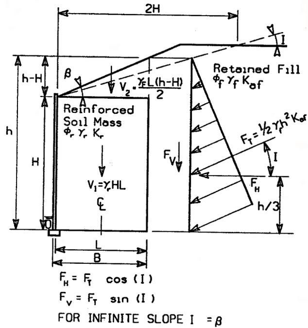
$K_o$  For Retained Fill Using  $\delta = \beta = I$
