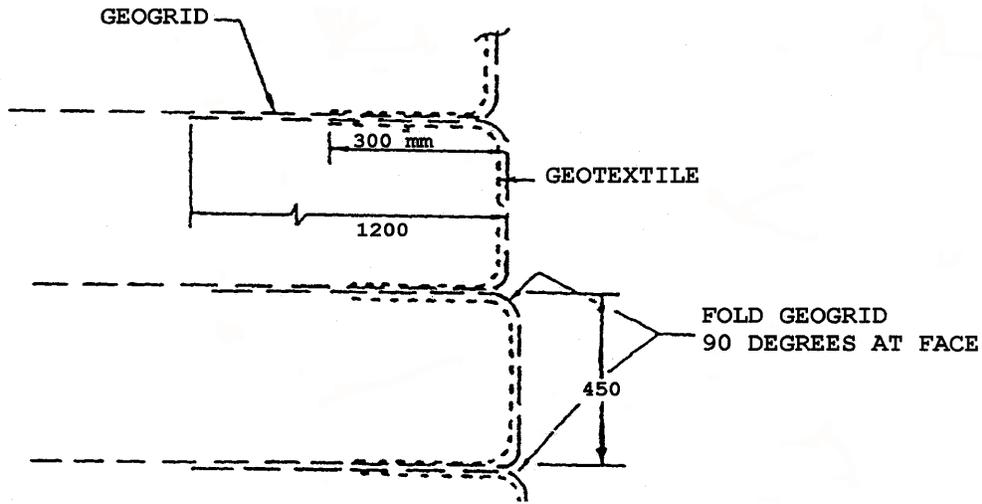
Figure 15. Typical geosynthetic face construction detail.
