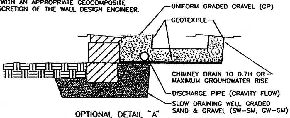
Figure 42. MBW drainage detail.
