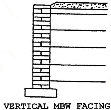
Figure 16. Types of geosynthetic reinforced soil wall facing.
