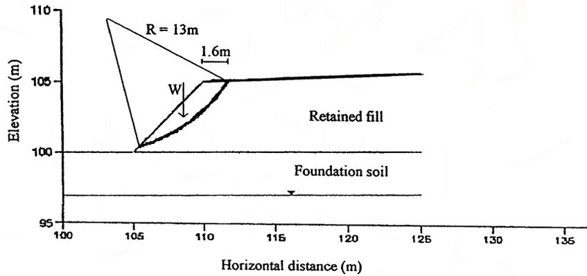
for  $R = 13\text{m}$ ,  $M_d = 1575\text{ kN/m}$
