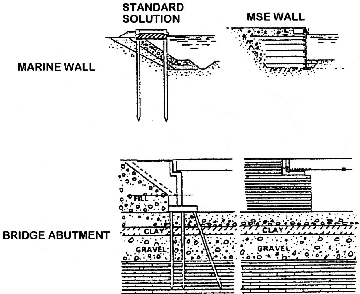
Figure 3. MSE wall applications, abutments, and marine.
