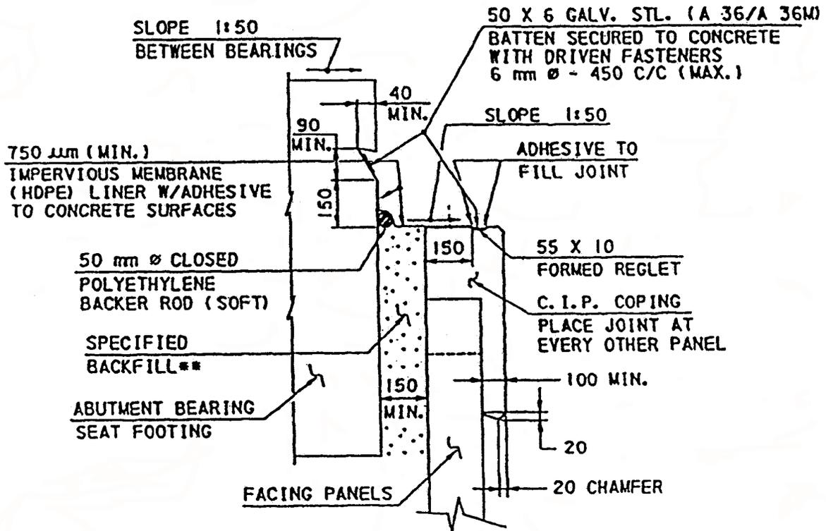
Figure 51. Abutment seat detail.
