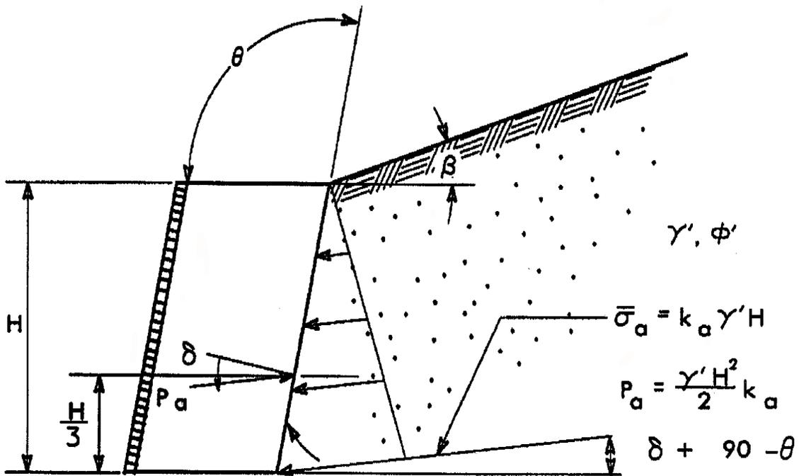
$$k_a = \frac{\sin^2 (\theta + \phi')}{\sin^2 \theta \sin (\theta - \delta) \left[ 1 + \sqrt{\frac{\sin (\phi' + \delta) \sin (\phi' - \beta)}{\sin (\theta - \delta) \sin (\theta + \beta)}} \right]^2}$$
