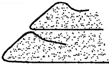
**OPTIONAL FACE CONSTRUCTION: OVER EXTEND FILL, COMPACT AND CUT BACK OR USE A FORM**
