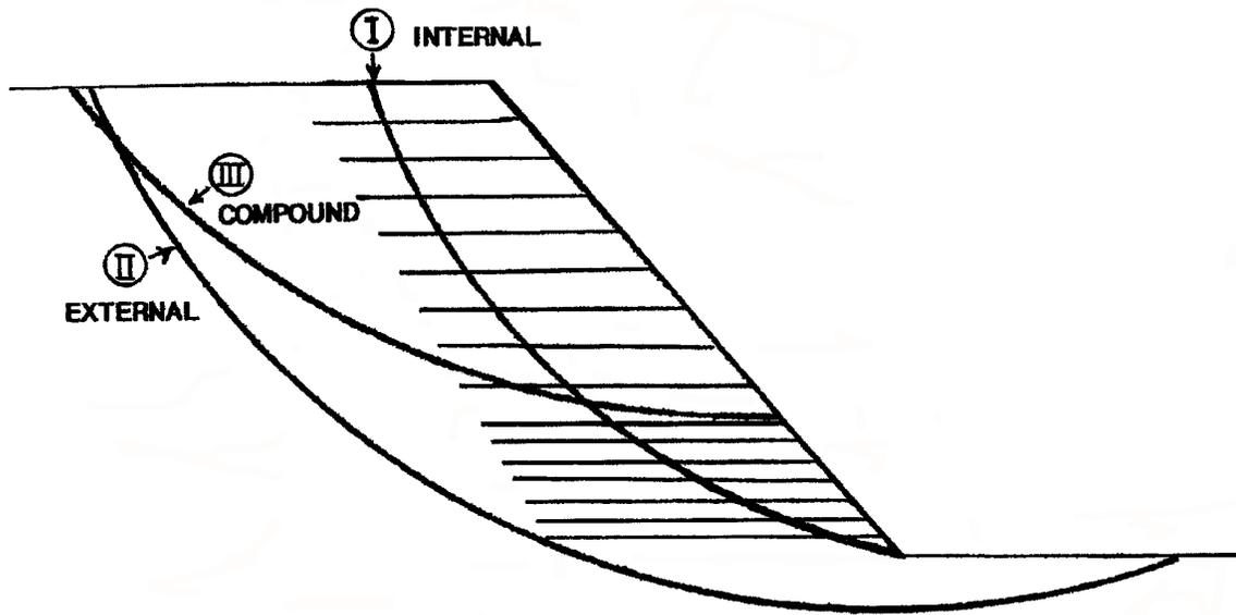
Figure 53. Failure modes for reinforced soil slopes.
