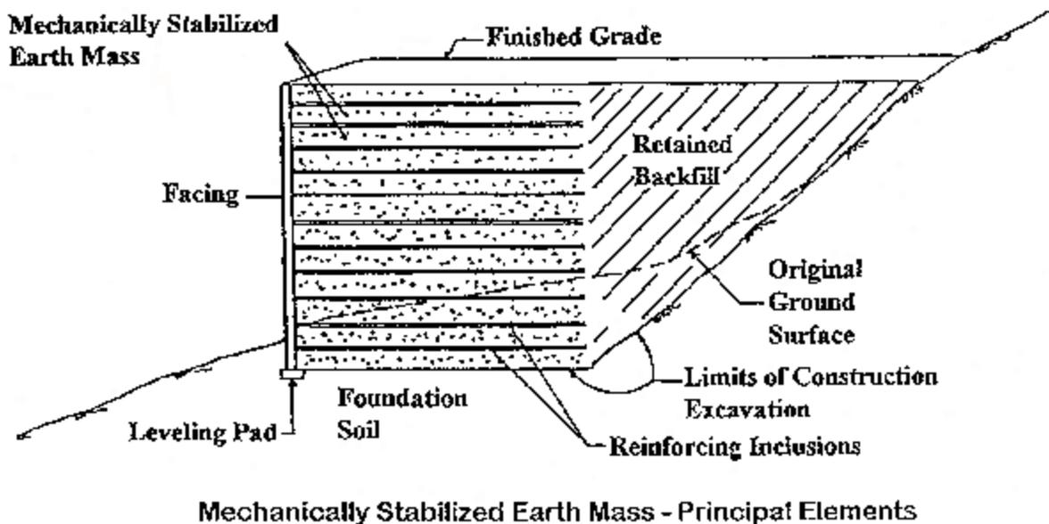
Figure 1. Generic cross section of a MSE structure.
