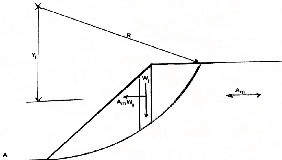
Figure 72. Seismic stability analysis.
