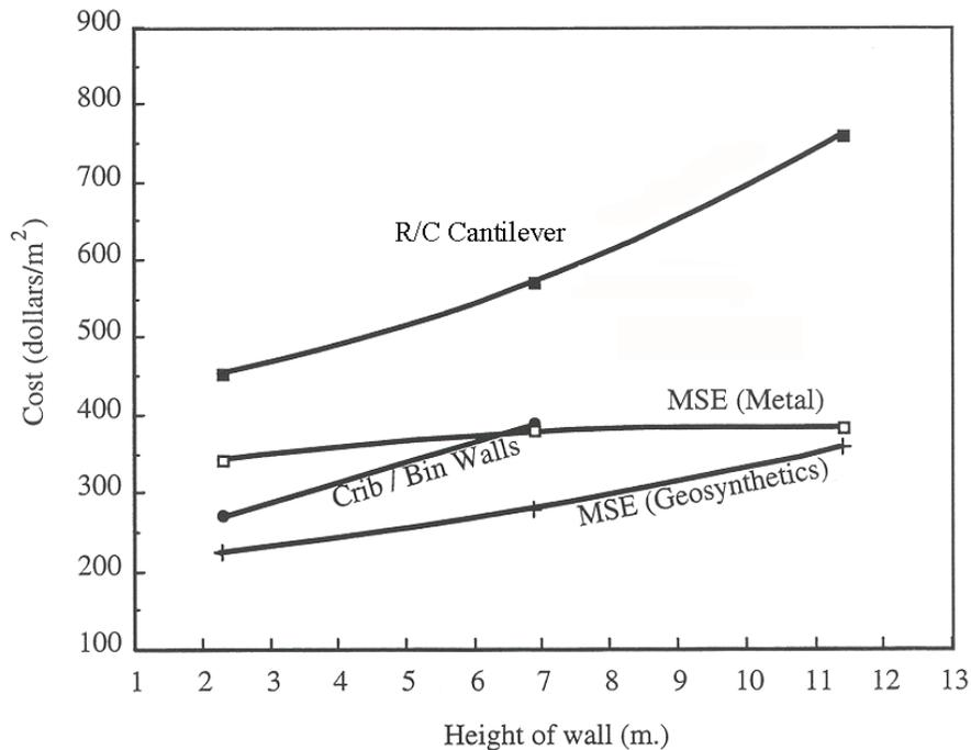
Figure 6. Cost comparison for retaining walls. <sup>(after 23)</sup>
