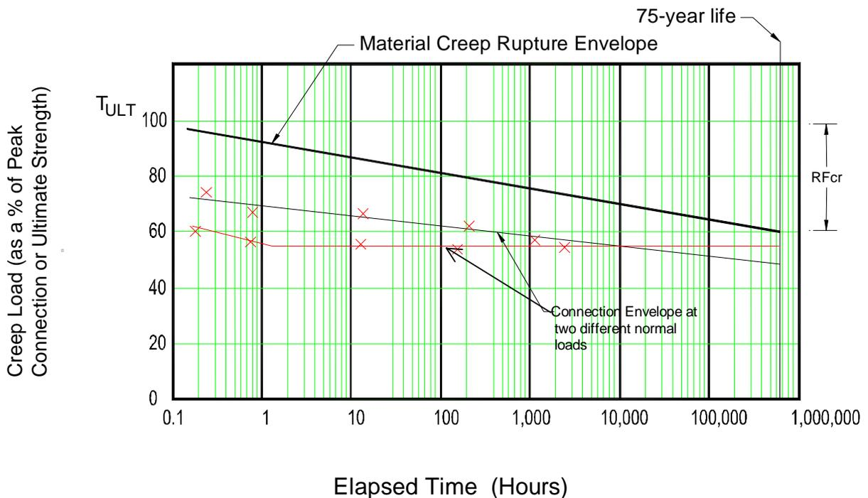
Figure A.5 Connection Strength Rupture Curve
