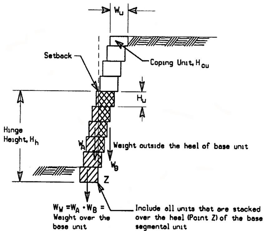
Hinge Height,  $H_h$ . The full weight of all segmental facing block units within  $H_h$  will be considered to act at the base of the lowermost segmental facing block.
